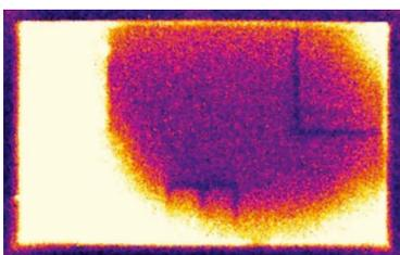
This IR image shows a large-area **delamination** in the sintered silver layer under a DCB substrate. Already a **delamination** of less than 1 mm diameter is clearly visible.
