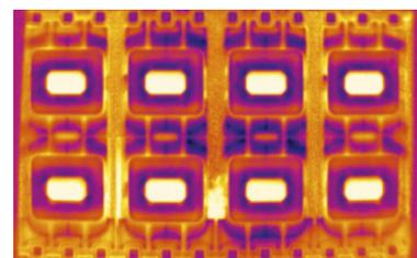
The investigation of **multiple components** at once can massively accelerate quality assessment. Visible defect sizes start at 500  $\mu\text{m}$ , depending on their vertical position.
