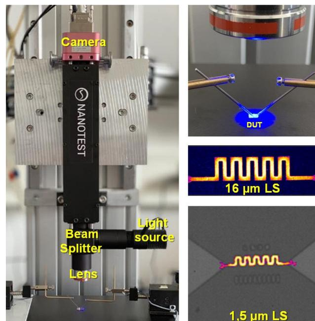
(1) **Reflective surfaces** are, by no means, measurable using infrared thermography without surface treatment. Thermorefectance, in contrary, allows thermographic studies of such samples without further treatment, like surface coating.
