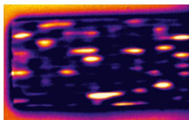
The **entrapped air** in a carbon fiber reinforced polymer caused by insufficient evacuation are visible as they affect the thermal performance. The **voids** sizes range between 0.5 and 2 mm.
