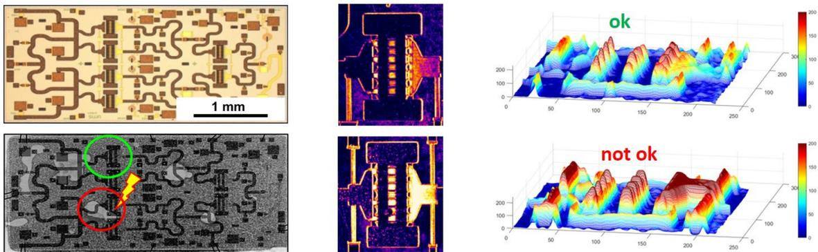
Thermo-reflectance imaging was used to locate hot spots in an HPA module. These hot spots can be caused by voids or cracks in the attach.
